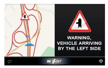
The warning algorithm, simultaneously with the turning on of the sign, activates the sending of warnings by I2V technologies to the vehicles that approach the crossroad in that direction.
